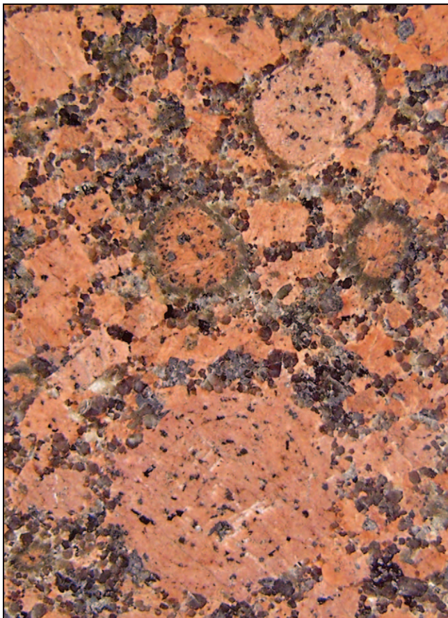
Figure 15. Rapakivi granite cladding Langford House (94).
